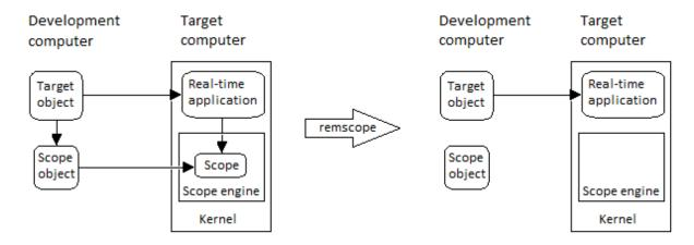
You can permanently remove only a scope that is added with the method addscope. This scope is outside the model. If you remove a scope that a scope block added inside the model, a subsequent run of that model recreates the scope.
