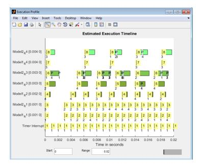
The Code Execution Profiling Report displays model execution profile results for each task.
