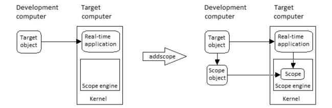
At the target computer command line, you can add a single target scope:
